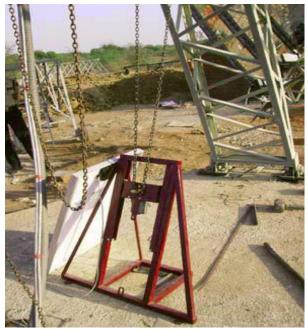
Fig: 3. Automatic tracking Stand for small Scheffler reflector
